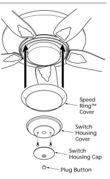
Figure 6e - Attaching Speed Ring™ Cover
